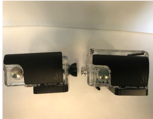
The photo above is a top-down view of the standard dive case (left) and the dive case after the addition of the BacPac (right)
