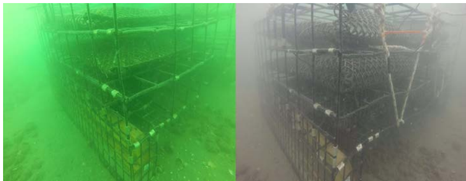
In the above photo, the image on the left was taken using a camera with no filter, and the image on the right was taken using a camera with the magenta filter
