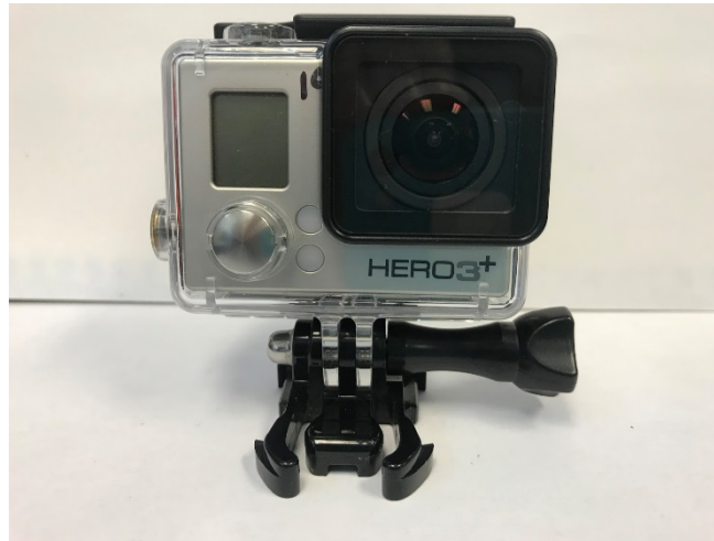
Pictured above is a Hero 3+ Silver camera in a 40 m dive case.
