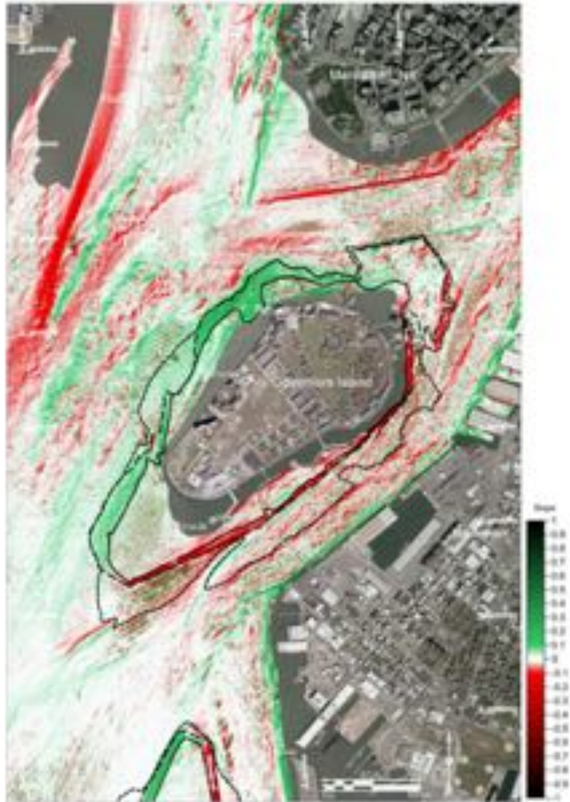
Figure 75. Bathymetric analysis for Governors Island (derivative maps for Area 2). Data from NOAA surveys H11353 (2004), H11395 (2006) and H11600 (2006) were combined in a 1m x 1m grid using a triangular linear interpolation. (Left) 2D first order derivative filter – slope. (Right) 2D second order derivative filter – change in slope.
