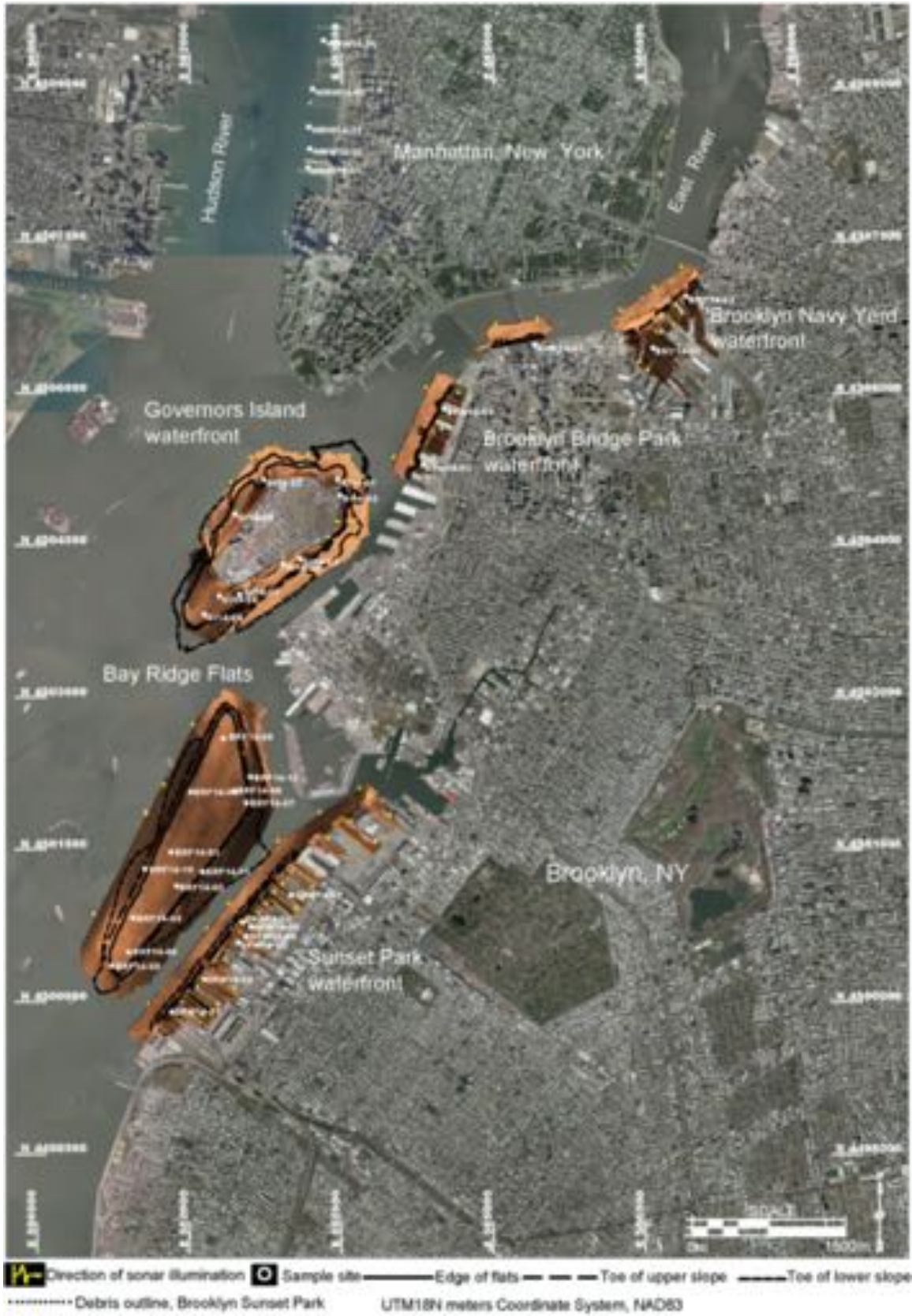
Figure 32. Side-scan orthosonograph of Brooklyn northwest including Governors Island insonified from the west.
