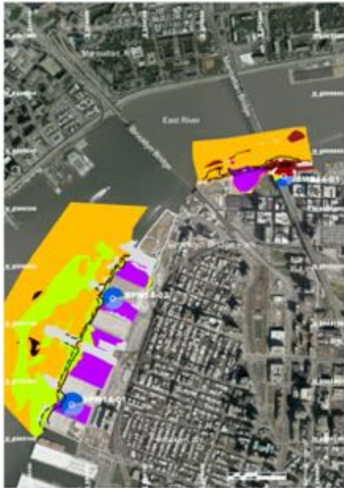
Figure 103. Bottom sediment type and geological substrate map for Brooklyn Bridge Park.
