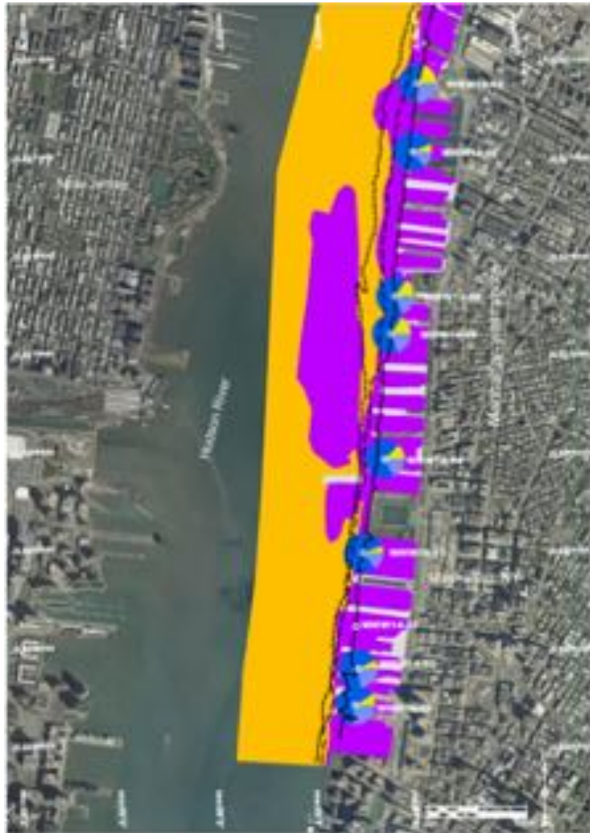
Figure 125. Bottom sediment type and geological substrate map for West Manhattan waterfront South.
