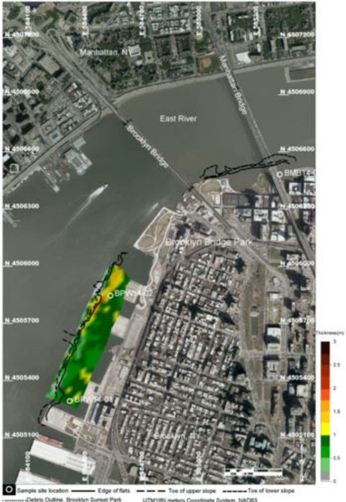
Figure 102. Acoustic silt isopach map for Brooklyn Bridge Park.
