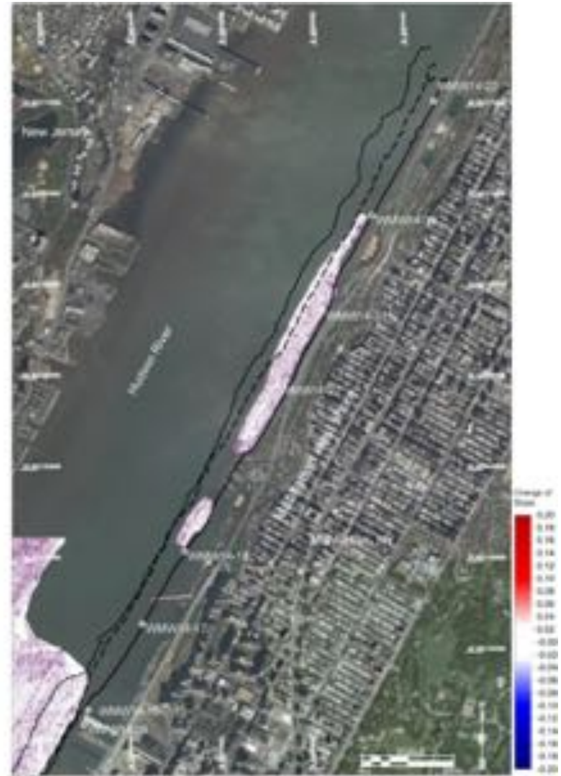
Figure 141. Bathymetric analysis for West Manhattan waterfront North (derivative maps for Area 8). Data from NOAA surveys F00573 (2009) and F00598 (2012) and USACE survey 4126 (2014) were combined in a 1m x 1m grid using a triangular linear interpolation. (Left) 2D first order derivative filter – slope. (Right) 2D second order derivative filter – change in slope.
