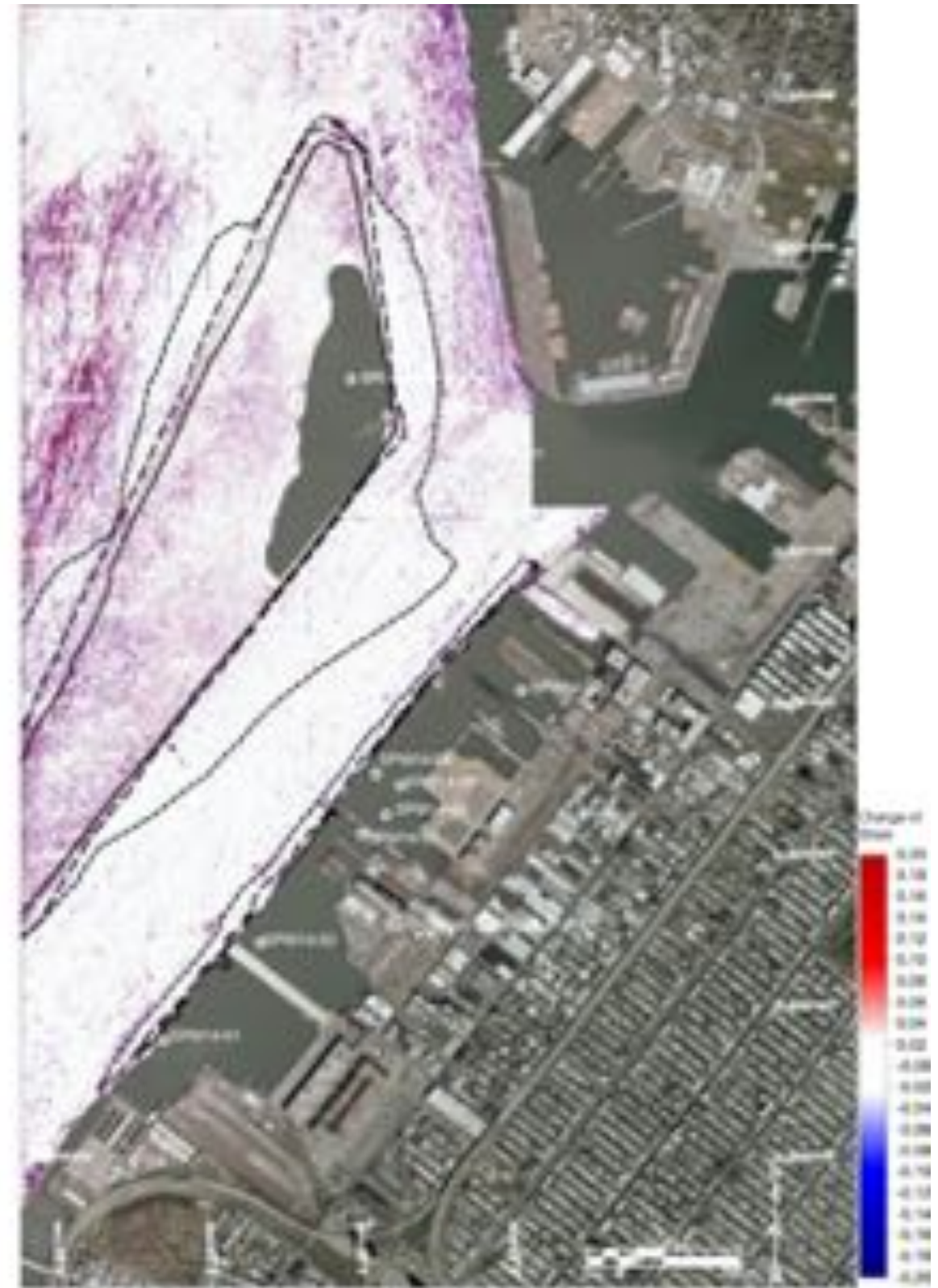
Figure 86. Bathymetric analysis for Sunset Park waterfront (derivative maps for Area 3). Data from NOAA survey H11600 (2006) were combined in a 1m x 1m grid using a triangular linear interpolation. (Left) 2D first order derivative filter – slope. (Right) 2D second order derivative filter – change in slope.
