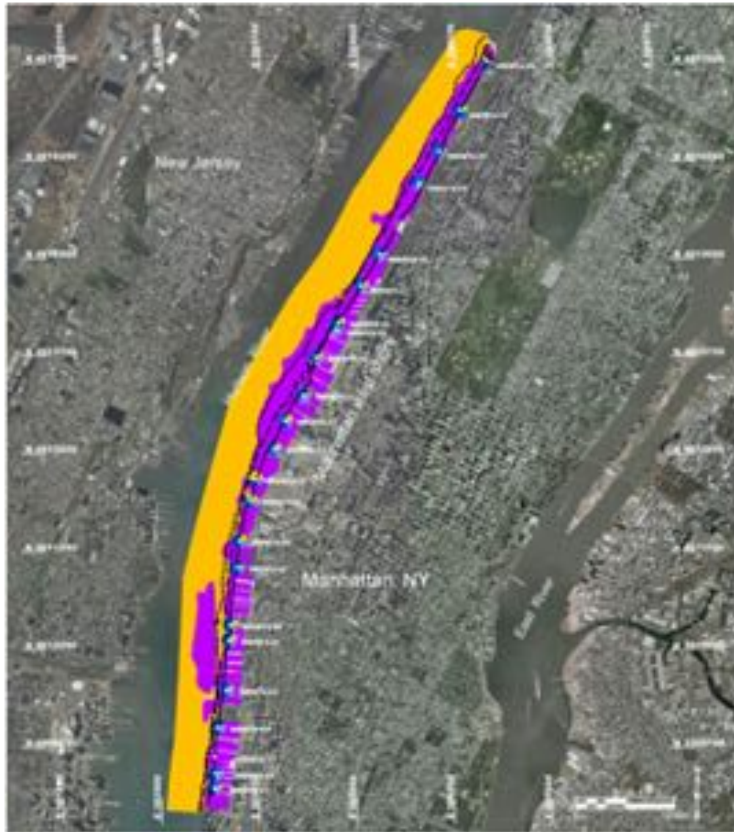
Figure 58. Bottom sediment type and geological substrate map for West Manhattan.
