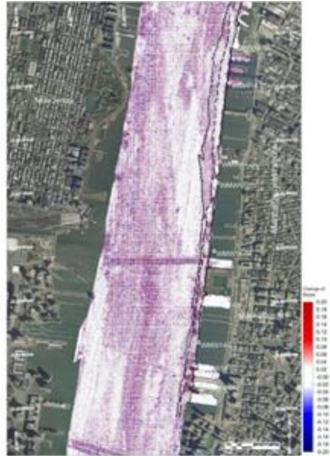
Figure 119. Bathymetric analysis for West Manhattan waterfront South (derivative maps for Area 6). Data from NOAA surveys F00573 (2009) and F00598 (2012) and USACE survey 4126 (2014) were combined in a 1m x 1m grid using a triangular linear interpolation. (Left) 2D first order derivative filter – slope. (Right) 2D second order derivative filter – change in slope.
