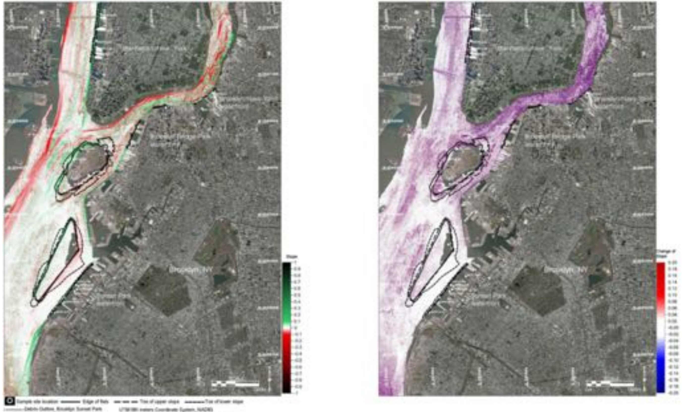
Figure 29. Derivative maps for 2006 composite bathymetry for Brooklyn northwest including Governors Island. Data from NOAA and USACE were combined in a 1m x 1m grid using a triangular linear interpolation. NOAA bathymetry includes surveys H10938 (1999), H11353 (2004), H11395 (2006) and H11600 (2006). USACE bathymetry includes survey 2676 (2004). (Left) 2D first order derivative filter – slope. (Right) 2D second order derivative filter – change in slope.
