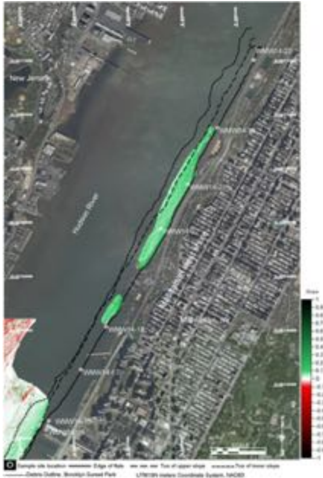
Figure 141. Bathymetric analysis for West Manhattan waterfront North (derivative maps for Area 8). Data from NOAA surveys F00573 (2009) and F00598 (2012) and USACE survey 4126 (2014) were combined in a 1m x 1m grid using a triangular linear interpolation. (Left) 2D first order derivative filter – slope. (Right) 2D second order derivative filter – change in slope.
