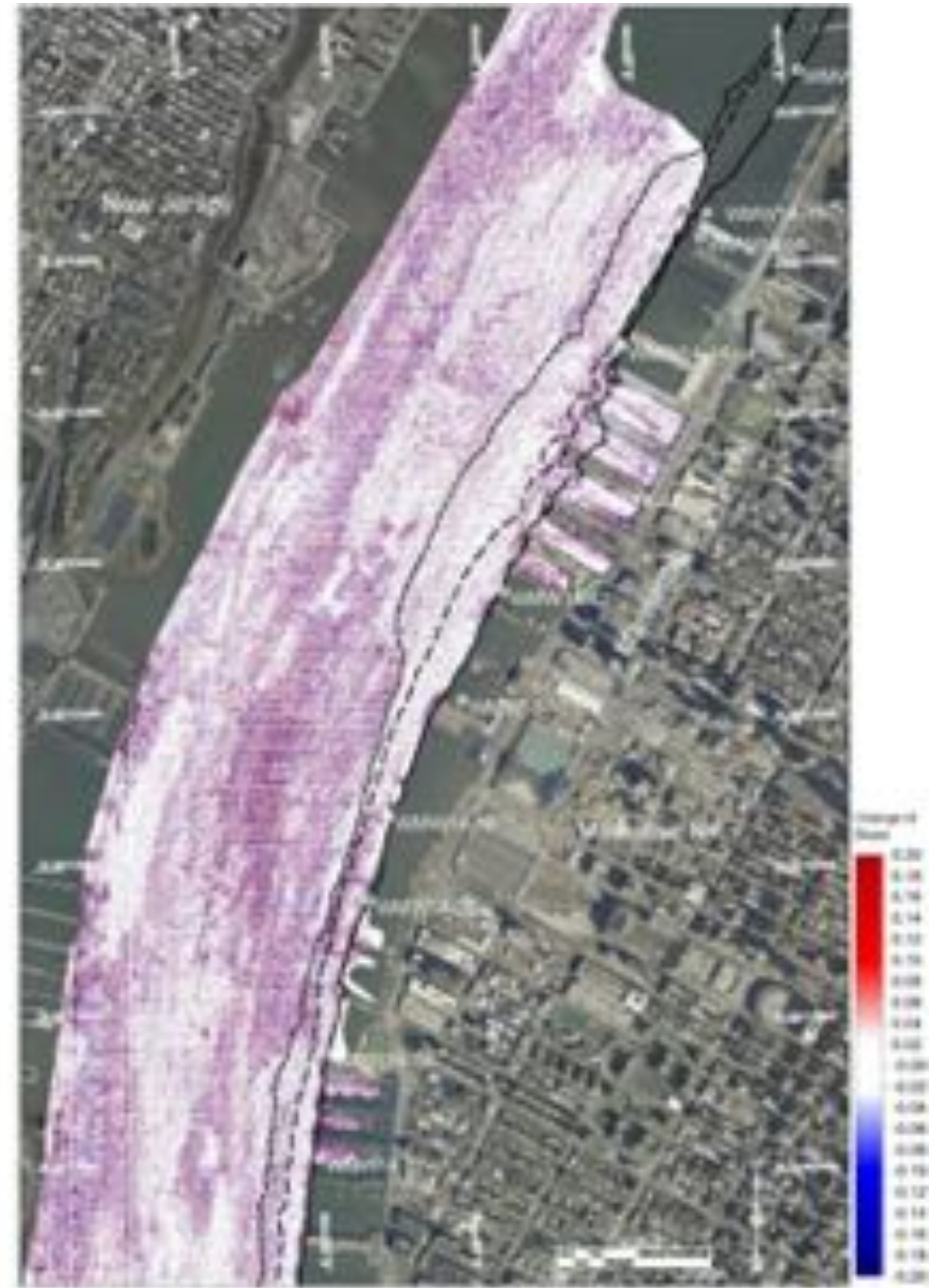
Figure 130. Bathymetric analysis for West Manhattan waterfront Middle (derivative maps for Area 7). Data from NOAA surveys F00573 (2009) and F00598 (2012) and USACE survey 4126 (2014) were combined in a 1m x 1m grid using a triangular linear interpolation. (Left) 2D first order derivative filter – slope. (Right) 2D second order derivative filter – change in slope.
