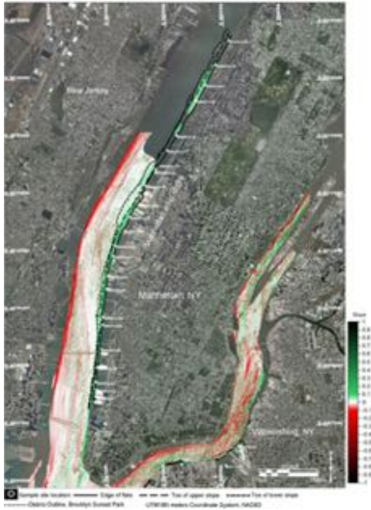
Figure 25. Derivative maps for 2014 composite bathymetry in Manhattan West shoreline. Data from NOAA and USACE were combined in a 1m x 1m grid using a triangular linear interpolation. NOAA bathymetry includes surveys F00573 (2009) and F00598 (2012). USACE bathymetry includes surveys 4069D (2013) and 4126 (2014). (Left) 2D first order derivative filter – slope. (Right) 2D second order derivative filter – change in slope.
