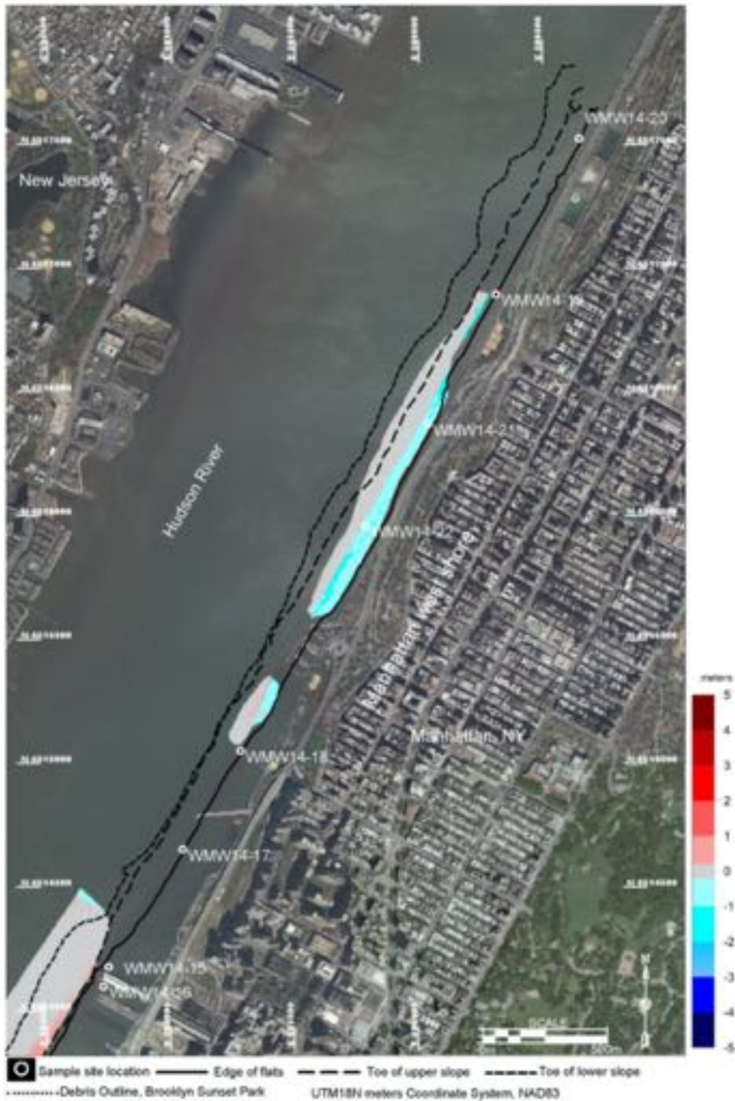
Figure 142. Bathymetry elevation difference map 2015 minus 2014 for West Manhattan waterfront North. The 2015 bathymetry includes single and multibeam bathymetries from e4sciences. The 2014 bathymetry includes NOAA surveys F00573 (2009) and F00598 (2012) and USACE survey 4126 (2014). The map displays both results of the difference in bathymetry for the 5m x 5m grid in the ultrashallow area, and the 1m x 1m grid in the deeper area. All grids were obtained with triangular linear interpolations.
