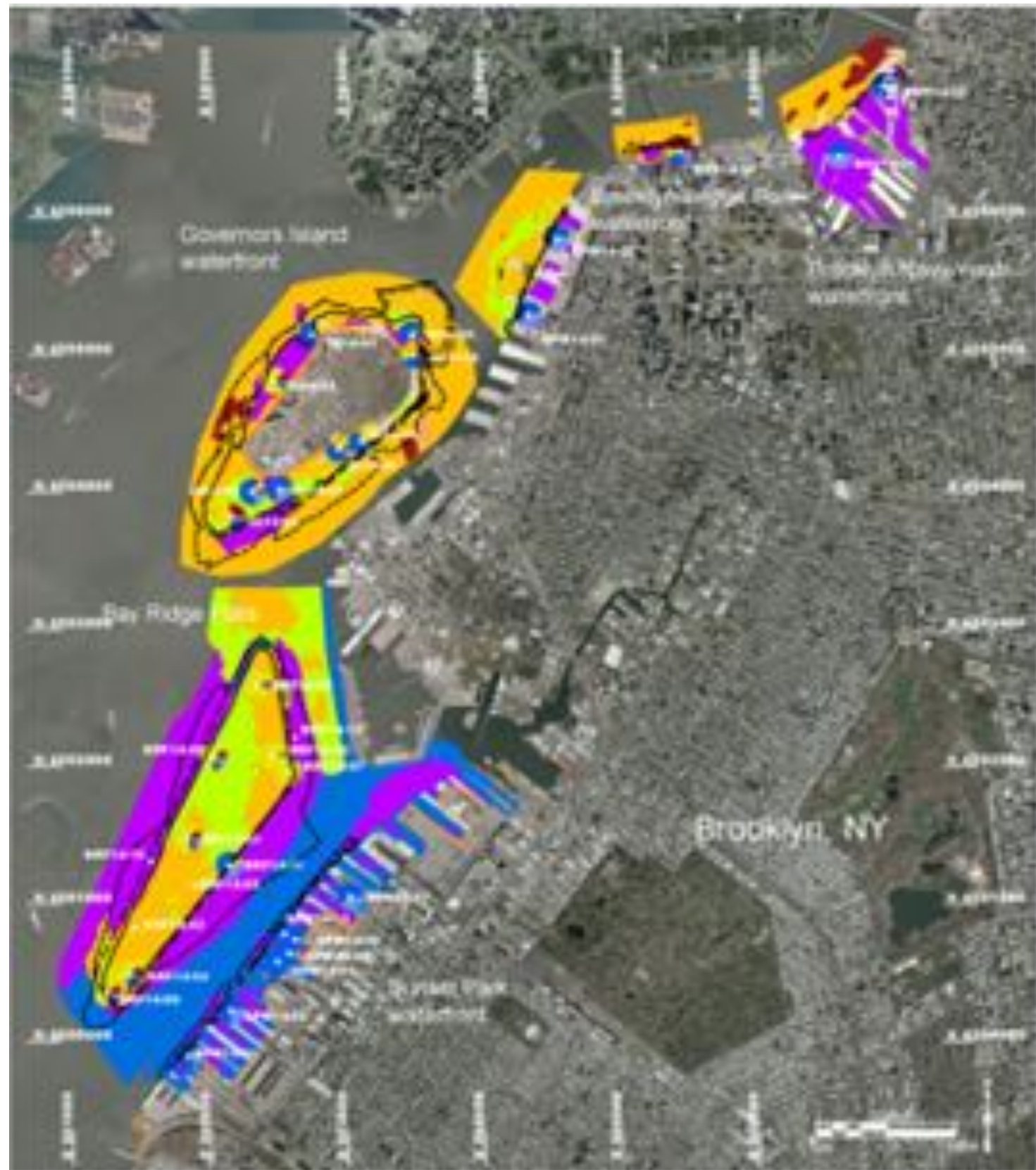
Figure 57. Bottom sediment type and geological substrate map for Brooklyn northwest including Governors Island.
