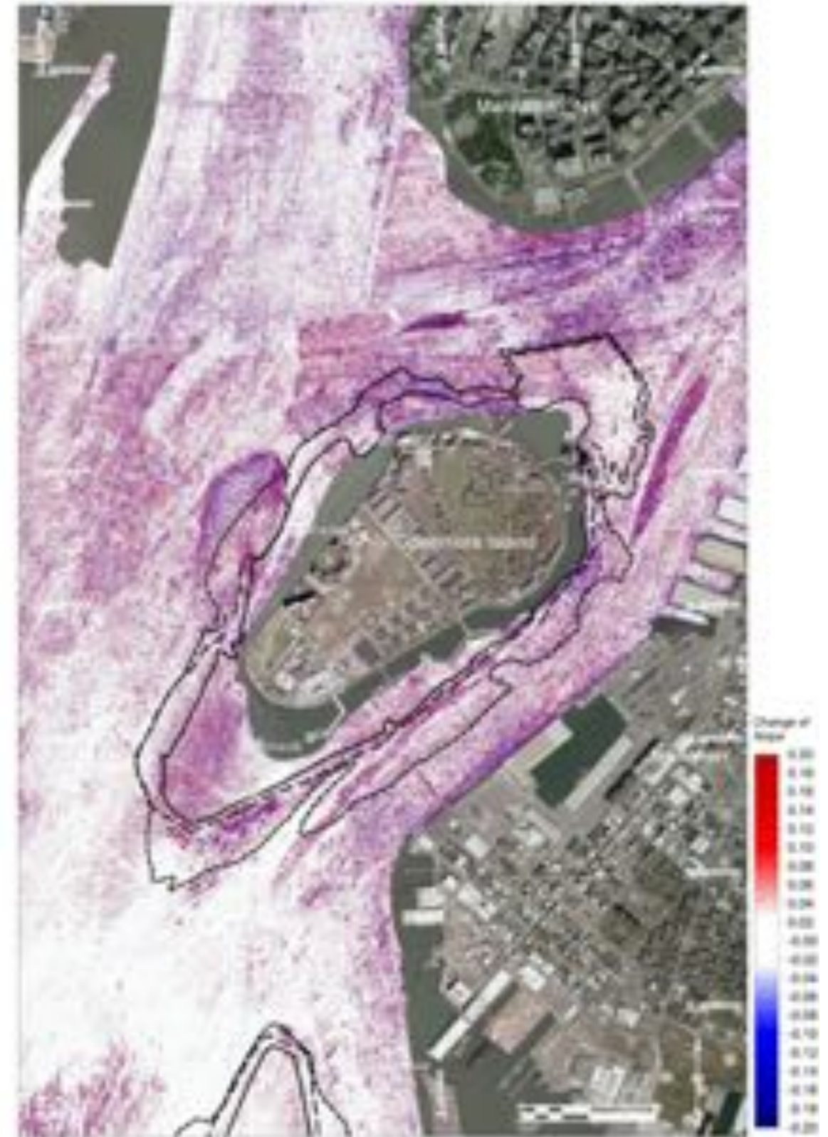
Figure 75. Bathymetric analysis for Governors Island (derivative maps for Area 2). Data from NOAA surveys H11353 (2004), H11395 (2006) and H11600 (2006) were combined in a 1m x 1m grid using a triangular linear interpolation. (Left) 2D first order derivative filter – slope. (Right) 2D second order derivative filter – change in slope.
