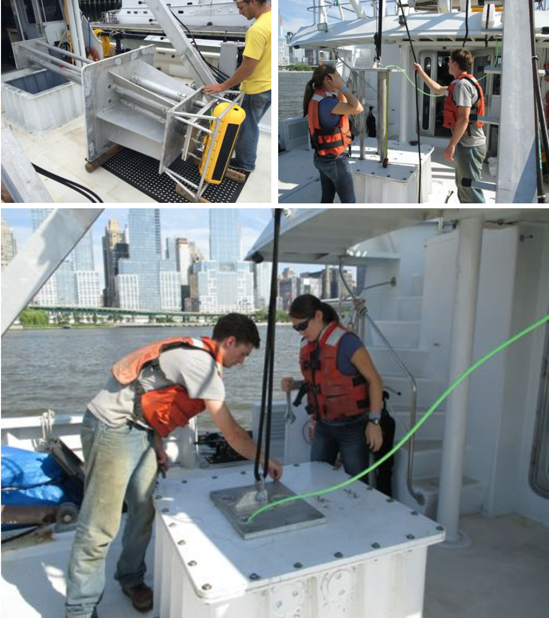
Figure 6. e4's Edgetech interferometric 6205 multibeam echosounder being set in place in the moon pool of the Time and Tide .
