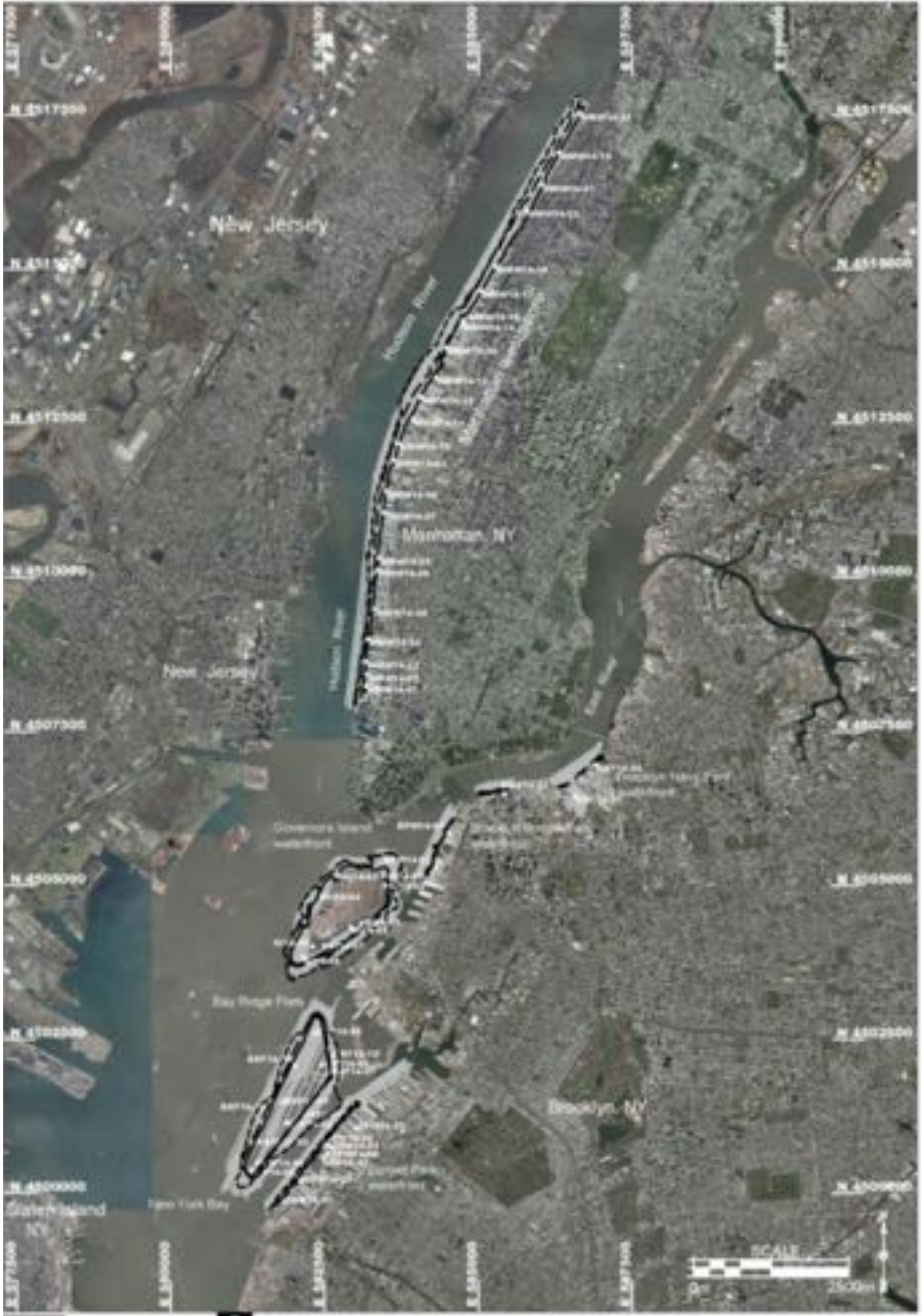
Figure 8. Coverage map for the bathymetry operations. Tracklines of the bathymetry appear in gray.
