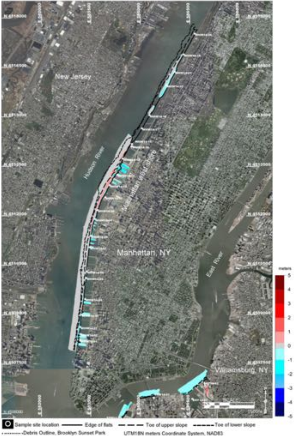
Figure 26. Difference map of bathymetry elevation 2015 minus 2014 bathymetry of West Manhattan. The 2015 bathymetry includes combined single and multibeam bathymetries from e4sciences. The 2014 bathymetry includes NOAA surveys F00573 (2009) and F00598 (2012) and USACE surveys 4069D (2013) and 4126 (2014). The map displays both results of the difference in bathymetry for the 5m x 5m grid in the ultrashallow area, and the 1m x 1m grid in the deeper area. All grids were obtained with triangular linear interpolations.
