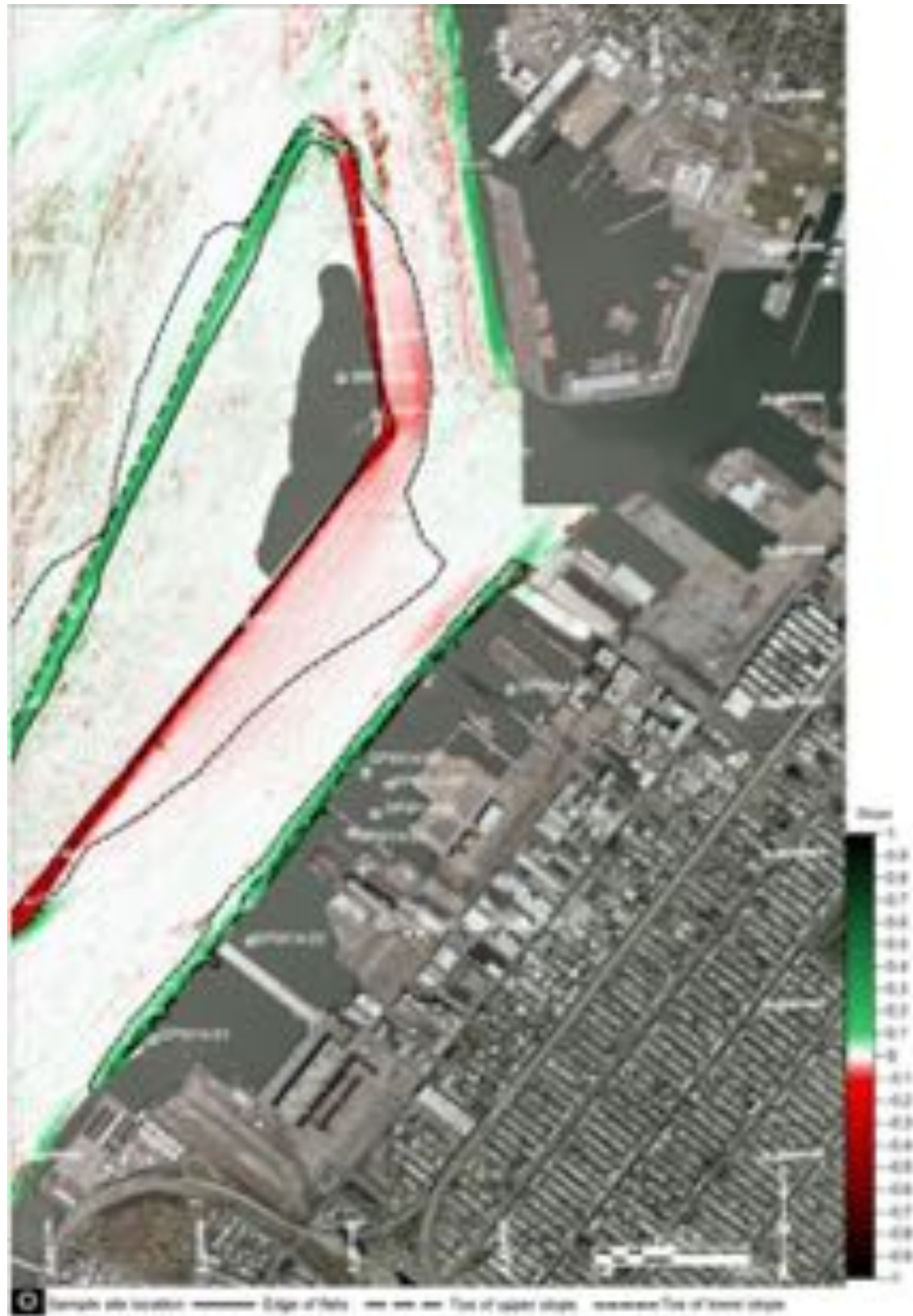
Figure 86. Bathymetric analysis for Sunset Park waterfront (derivative maps for Area 3). Data from NOAA survey H11600 (2006) were combined in a 1m x 1m grid using a triangular linear interpolation. (Left) 2D first order derivative filter – slope. (Right) 2D second order derivative filter – change in slope.
