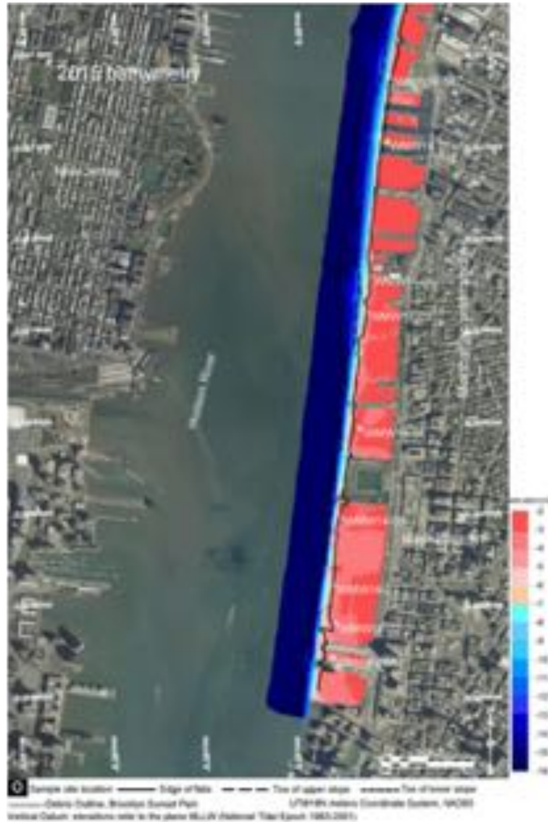
Figure 118. Bathymetric and location map for West Manhattan waterfront South. (Left) Single and multibeam data from e4sciences (2015) were combined in 5m x 5m and 1m x 1m grids, respectively, using a triangular linear interpolation. (Right) Historical data from NOAA surveys F00573 (2009) and F00598 (2012), and USACE survey 4126 (2014), were combined in a 1m x 1m grid using a triangular linear interpolation.
