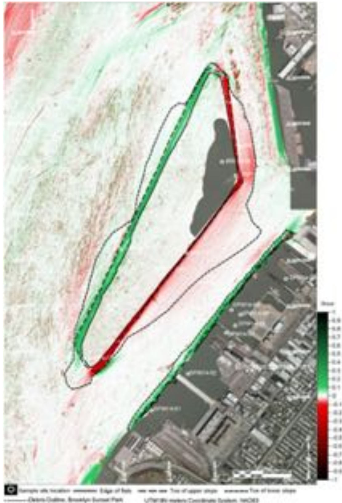
Figure 64. Bathymetric analysis for Bay Ridge Flats (derivative maps for Area 1). Data from NOAA survey H11600 (2006) were combined in a 1m x 1m grid using a triangular linear interpolation. (Left) 2D first order derivative filter – slope. (Right) 2D second order derivative filter – change in slope. The NOAA survey H11600 was incomplete in the shallowest water.
