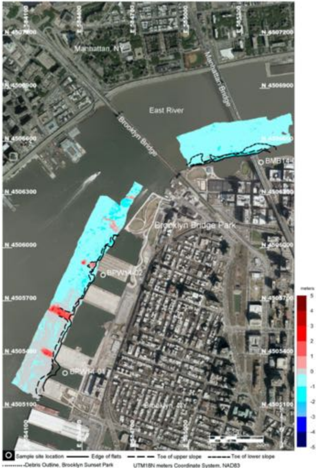
Figure 98. Bathymetry elevation difference map 2015 minus 2006 for Brooklyn Bridge Park. The 2015 bathymetry includes single and multibeam bathymetries from e4sciences. The 2006 bathymetry includes NOAA survey H11353 (2004). The map displays both results of the difference in bathymetry for the 5m x 5m grid in the ultrashallow area, and the 1m x 1m grid in the deeper area. All grids were obtained with triangular linear interpolations.
