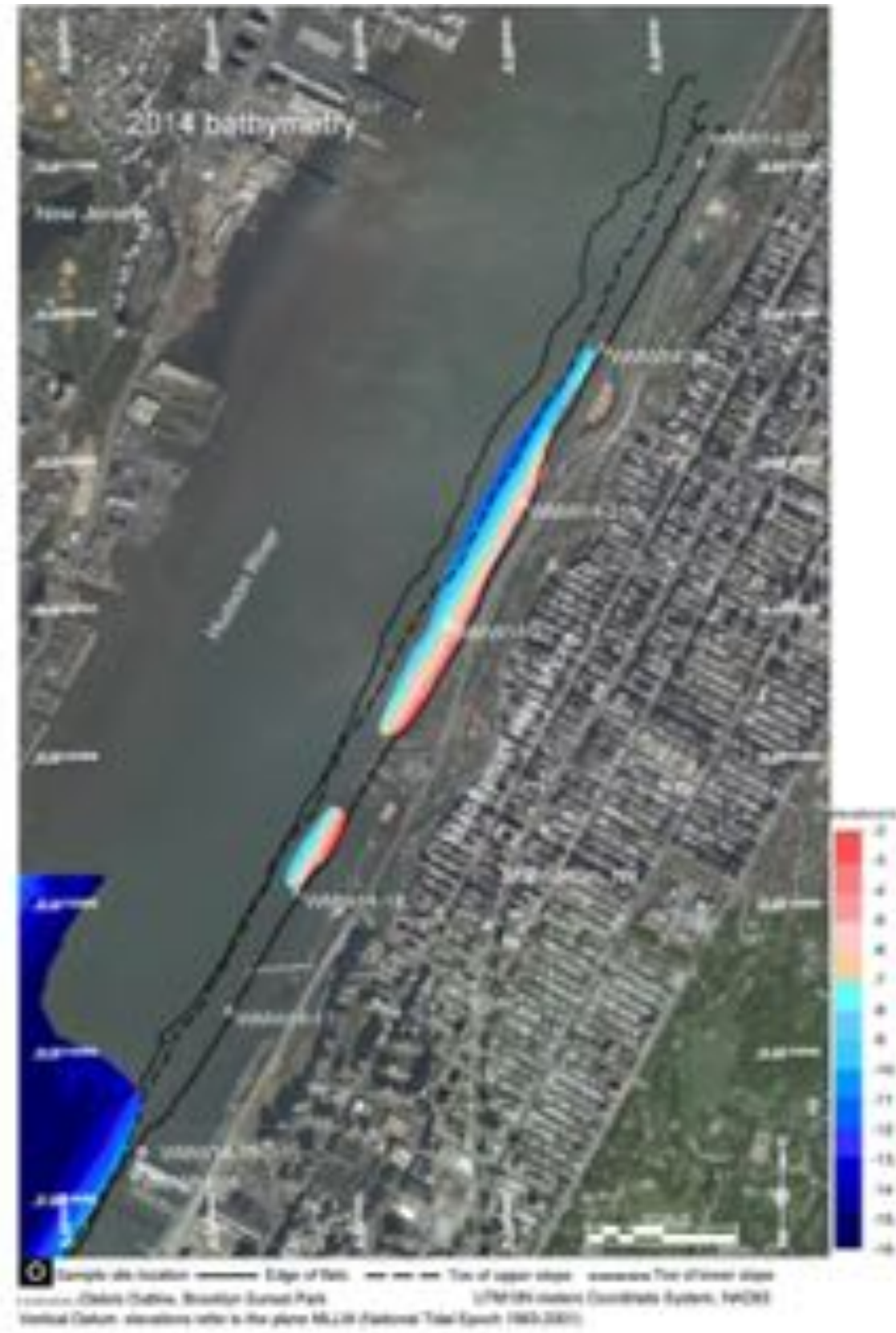
Figure 140. Bathymetric and location map for West Manhattan waterfront North. (Left) Single and multibeam data from e4sciences (2015) were combined in 5m x 5m and 1m x 1m grids, respectively, using a triangular linear interpolation. (Right) Historical data from NOAA surveys F00573 (2009) and F00598 (2012), and USACE survey 4126 (2014), were combined in a 1m x 1m grid using a triangular linear interpolation.
