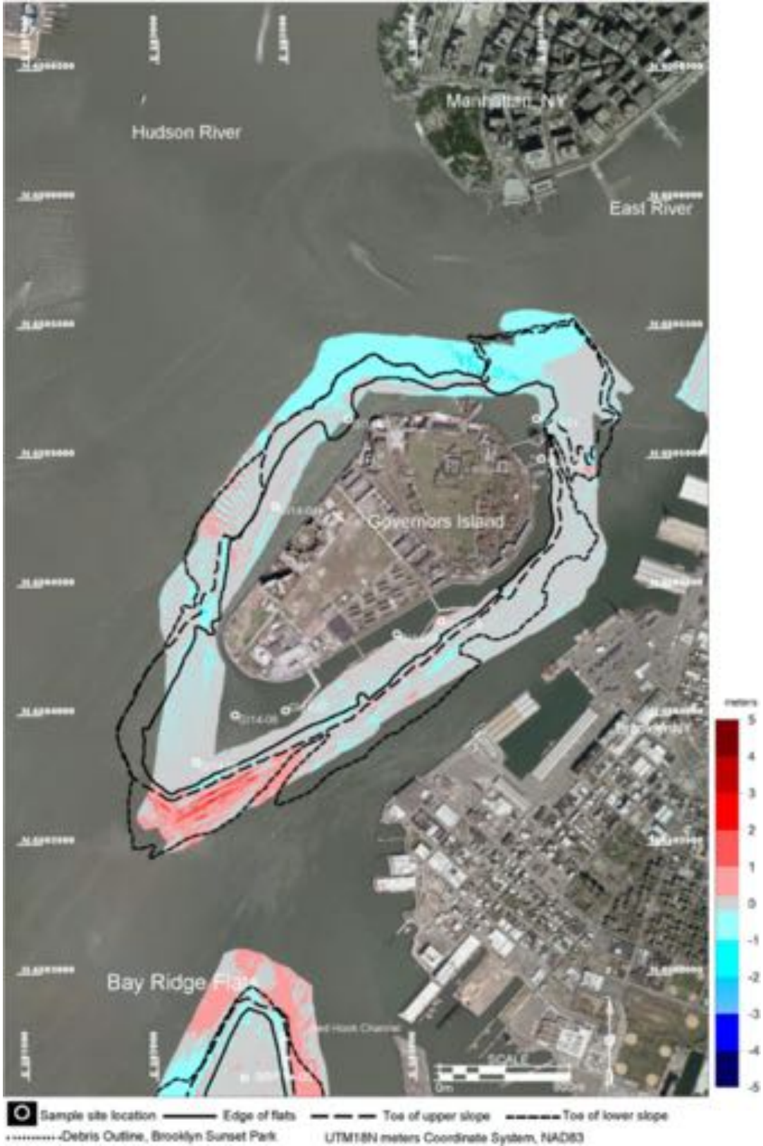
Figure 76. Bathymetry elevation difference map 2015 minus 2006 for Governors Island. The 2015 bathymetry includes multibeam bathymetry from e4sciences. The 2006 bathymetry includes NOAA survey H11600. Data were combined in a 1m x 1m grid using a triangular linear interpolation.
