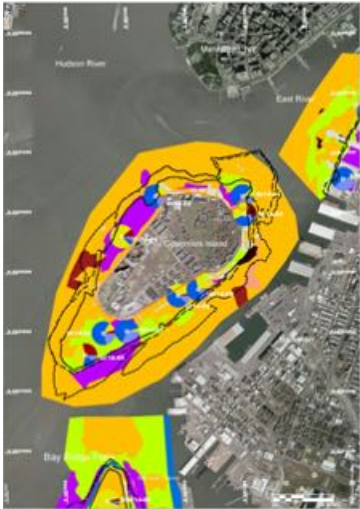
Figure 81. Bottom sediment type and geological substrate map for Governors Island.
