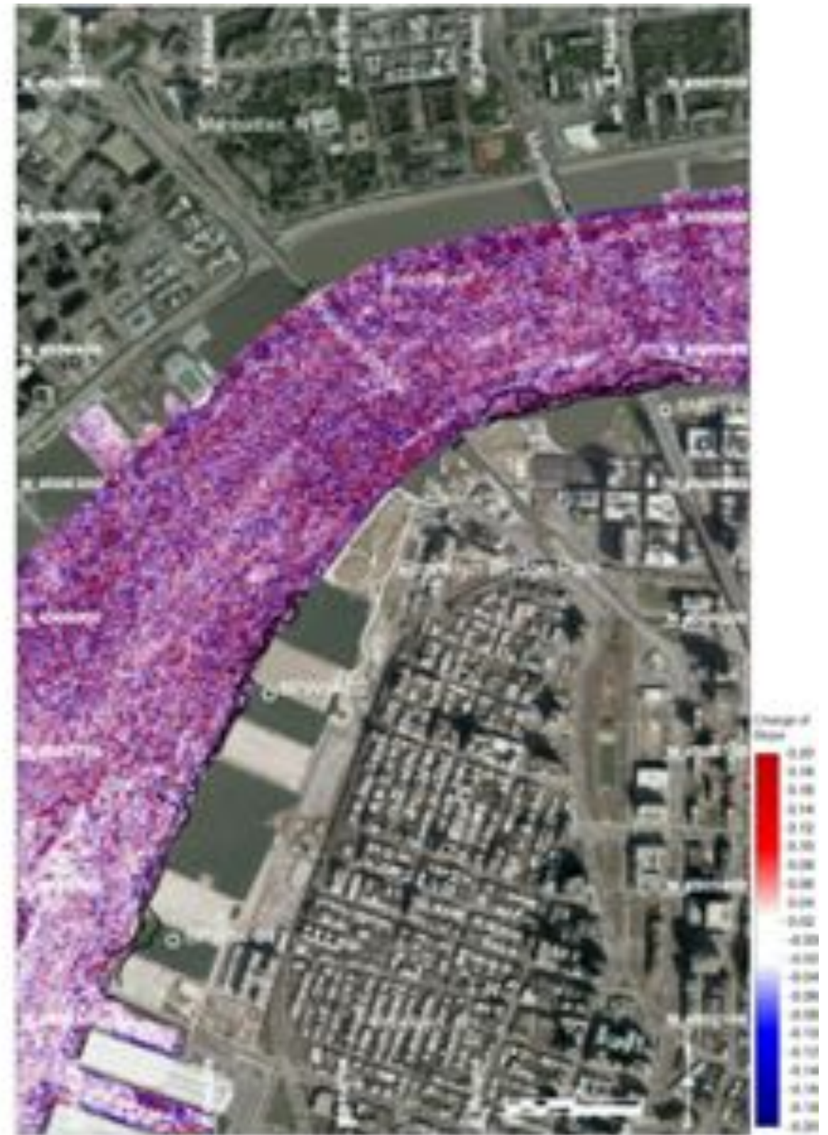
Figure 97. Bathymetric analysis for Brooklyn Bridge Park (derivative maps for Area 4). Data from NOAA survey H11353 (2004) were combined in a 1m x 1m grid using a triangular linear interpolation. (Left) 2D first order derivative filter – slope. (Right) 2D second order derivative filter – change in slope.
