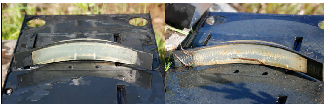
Figure 11 Photo of the DIDSON lens: clean (left) and covered by drifting pollen (right) (Lilja et al. 2010).
