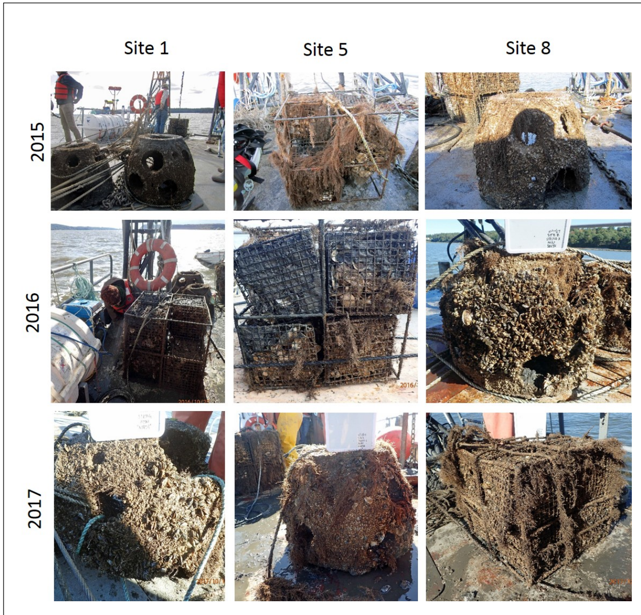
Fig. 2. Retrieval of test substrates by year and site. Note damaged gabions all three years.
