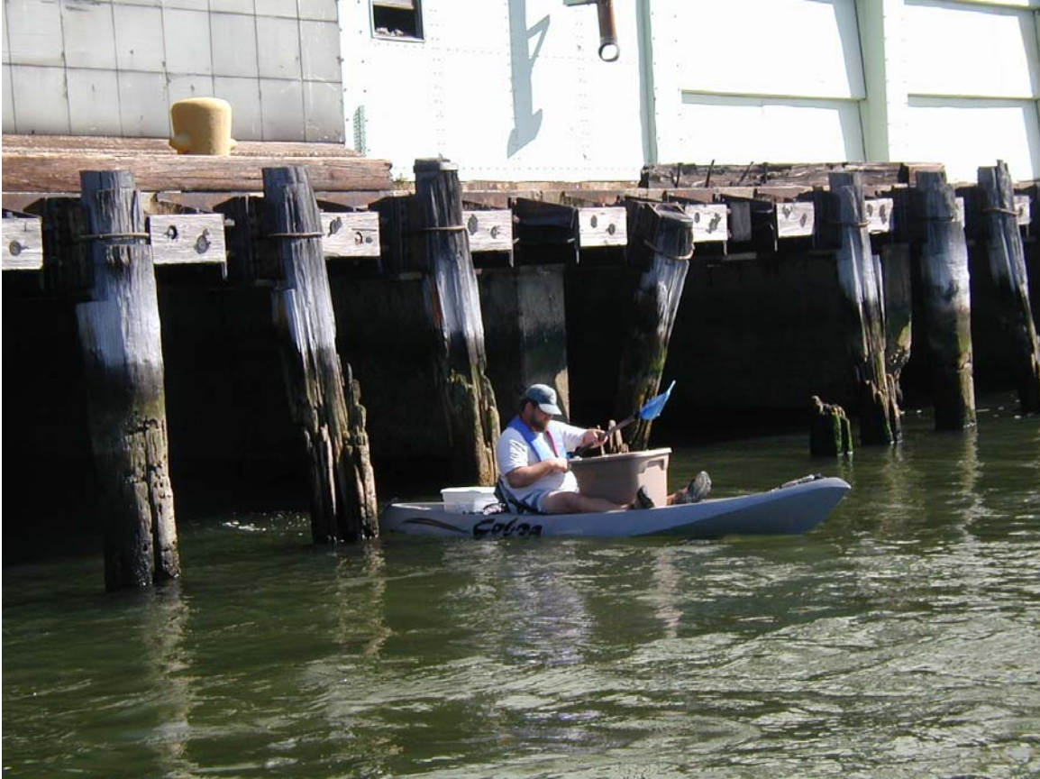
Figure 2. A Rutgers University scientist emerges from under Pier 57 during a DIDSON survey. The DIDSON is mounted under the kayak bow, batteries are behind the paddler, and the laptop is inside the spray guard/sunshade ahead of the paddler. The kayak is very quiet and able to enter shallow water without disturbing nearby fish.
