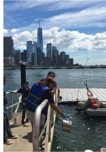
Fig. 10 | Interns gathering benthic sediment samples at Pier 40 via Eckman dredge.
