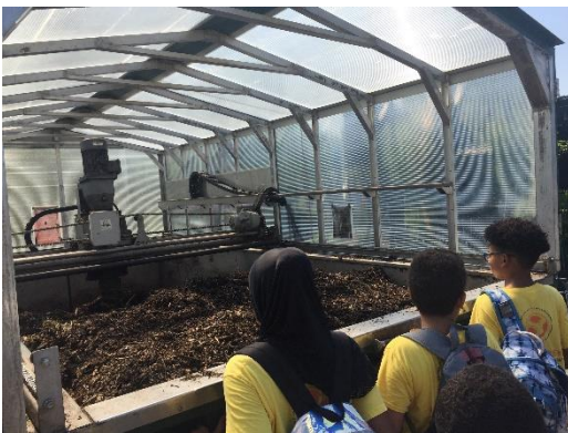
Fig. 1 (left) | Students learn how organic waste is collected at HRPK’s compost center and processed in an aerating vessel in order to produce compost.
